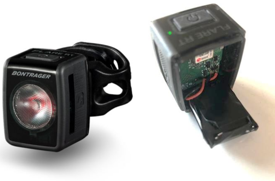
Figure 4. The Flare RT bike light (above left), rebuilt with B2V GNSS and Bluetooth chipset (above right).
