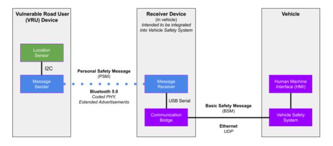
A VRU device was created that accesses information from its GNSS device and packages it into a PSM and advertises it over Bluetooth 5 with Coded PHY and Extended Advertisements. A second device receives each PSM, constructs a BSM and sends it to a vehicle ADAS system using an existing ethernet interface. Message communication is one-way, from VRU to vehicle. The VRU does not receive nor process any data from the vehicle.
