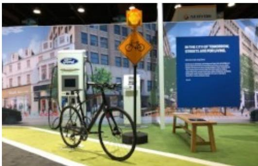
Our latest addition to the B2V program is a cyclist detection sign that blinks whenever a cyclist is nearby while also sending a wireless signal to connected vehicles over C-V2X. The team debuted the tech in the Ford booth at [SAE World Congress](#).
